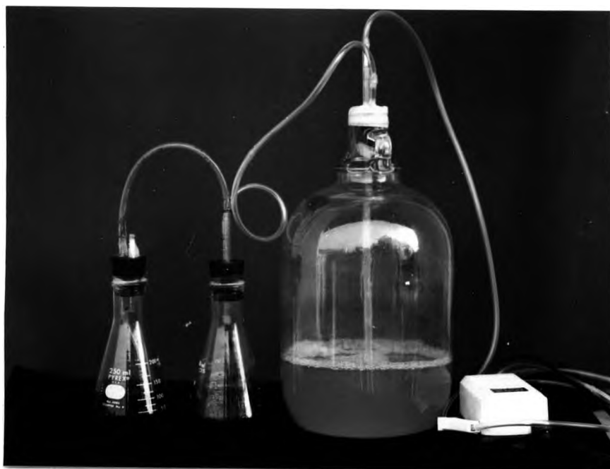
Figure 3.2 Bacterial culture and trap solution for determined volatilization Of mercury
