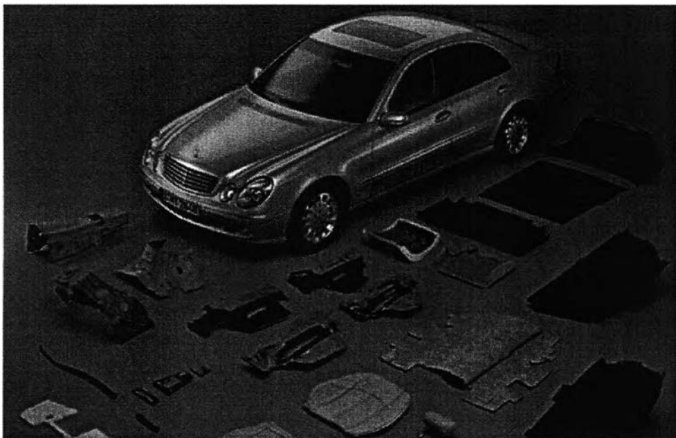
Figure 2.2 Flax, hemp, sisal, wool and other natural fibers used in 50 Mercedes–Benz E–Class components (James H. et al. 2006).
