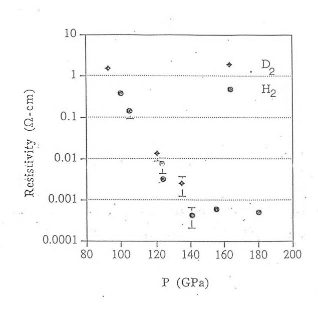
Figure 1.1 The metallic phase of liquid hydrogen has initially occurred at Pressure 140 GPa and temperature 3000 Kelvin taken from [6].
