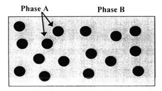
**Figure 1.1** Schematic drawing of a mixed matrix membrane – phase A dispersed in phase B matrix.
