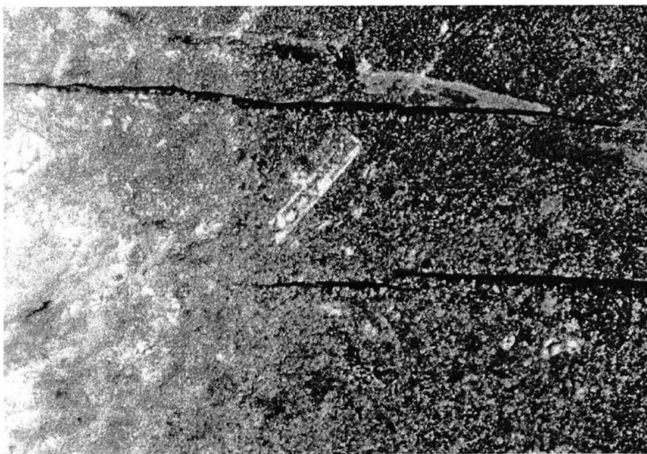
Figure 3.34 The photomicrograph of fossiliferous micrite in the lower part of picture, and microcrystalline chert in the middle and upper parts of picture, of the lithofacies V. (Crossed nicols, x44)
