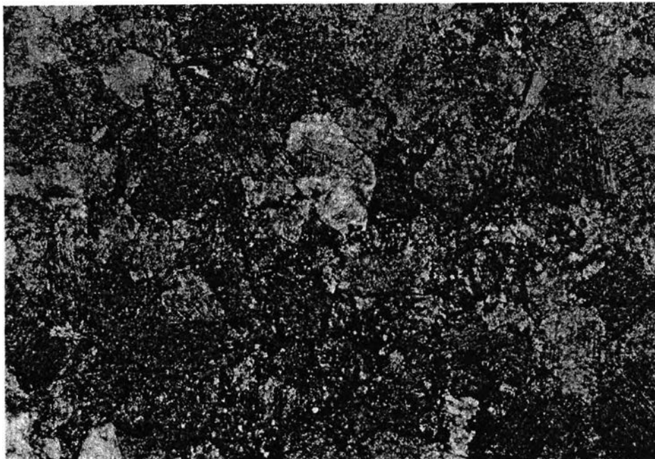
Figure 3.24 The photomicrograph of sorted biosparite of the lithofacies III showing closely packed of carbonate allochems which cemented by sparry calcite with some micrite infilled between carbonate grains. (Crossed nicols, x44)
