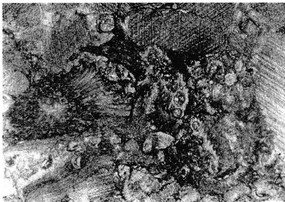
Figure 3.22 The photomicrograph of crinoidal biosparite of the lithofacies II showing fragments of bryozoa and other skeletal remains cemented by sparry calcite. (Crossed nicols, x44)
