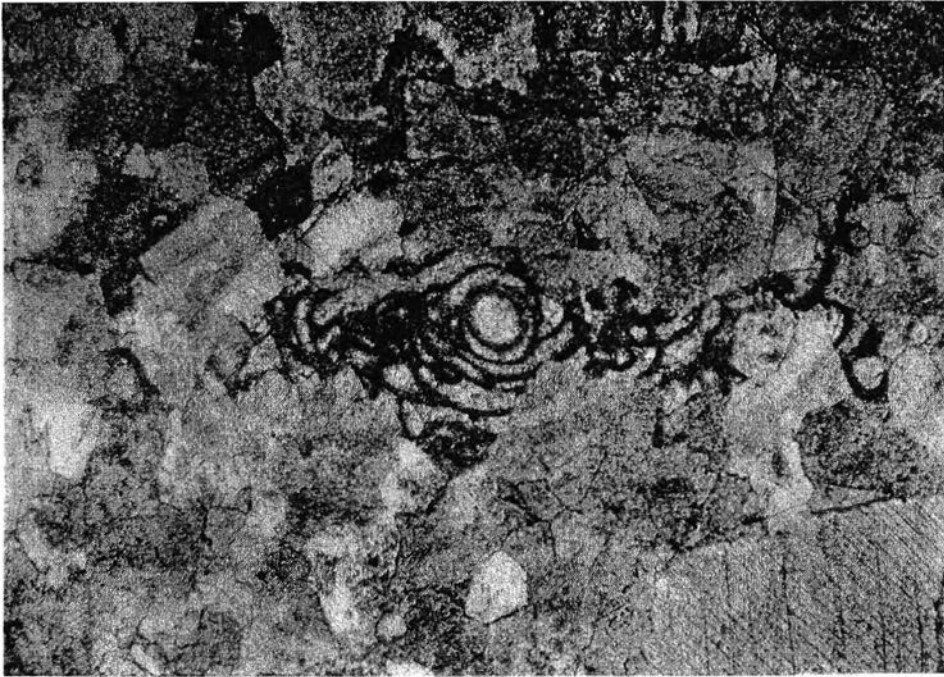
Figure 3.28 The photomicrograph of dolomitic calcarenite of the lithofacies IV showing the dolomite rhombs cut across the foraminiferal test. (Crossed nicols, x44)
