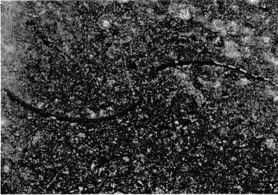
Figure 3.17 The photomicrograph of sparse biomicrite of the lithofacies I showing sparse organic skeletons embedded in micrite. (Crossed nicols, x44)
