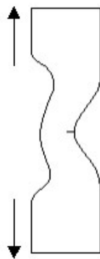
Figure 3.8 Tear specimen type C according to ISO 34
