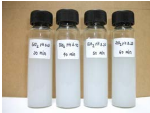
Figure 4.1 Physical appearance of the 1wt% silica aqueous suspension at different ultrasonic times
