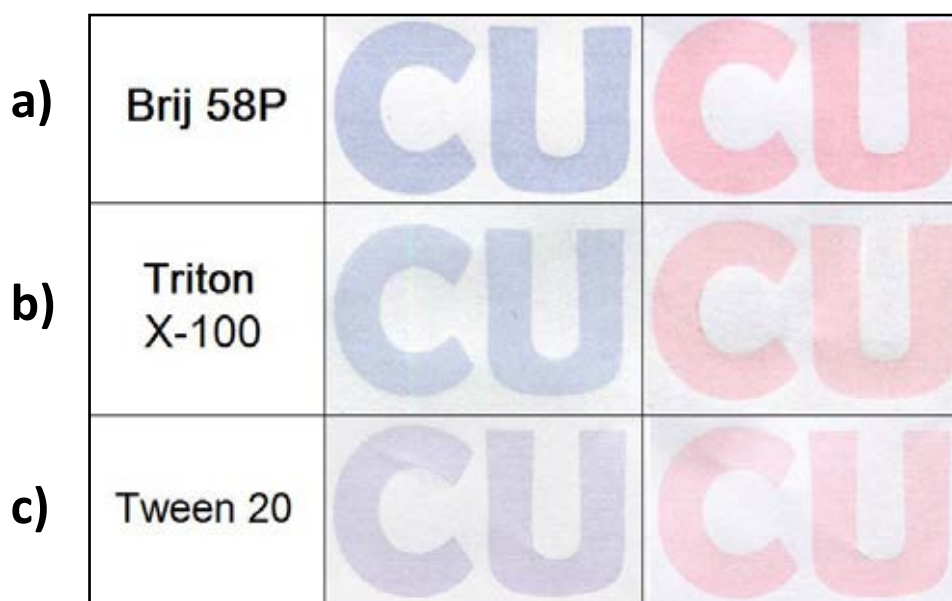
Figure 3.2 Color images of poly(PCDA) printed from PCDA/surfactant aqueous solutions using a) Brij ® 58P b) Triton ® X-100 c) Tween ® 20 before (left) and after (right) heating at 90 °C for 10 sec.
