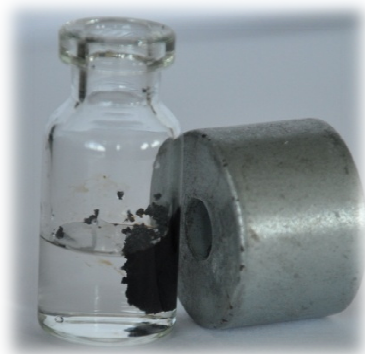
Figure 4.22 Composite is removed by permanent magnet.
