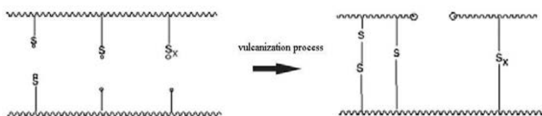
Figure 2.5 Example of vulcanization process.
