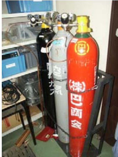
Fig 3-26 Oxygen, Air and hydrogen tanks
