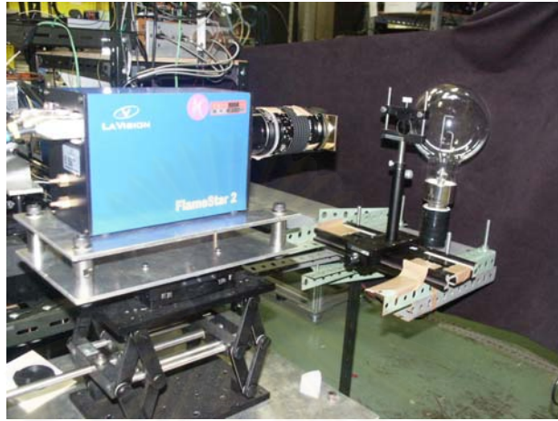
Fig 4-11 Calibration experiment for two color method
