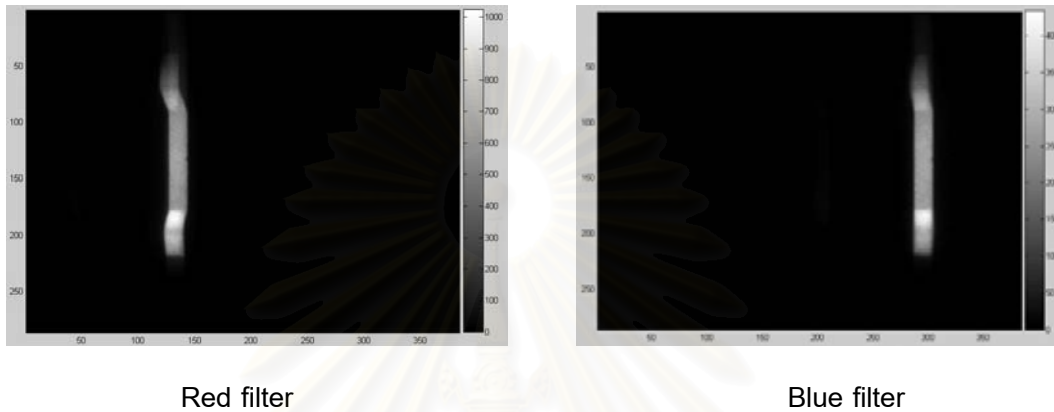
Fig 4-12 Tungsten ribbon intensity distribution at 1600 °C
