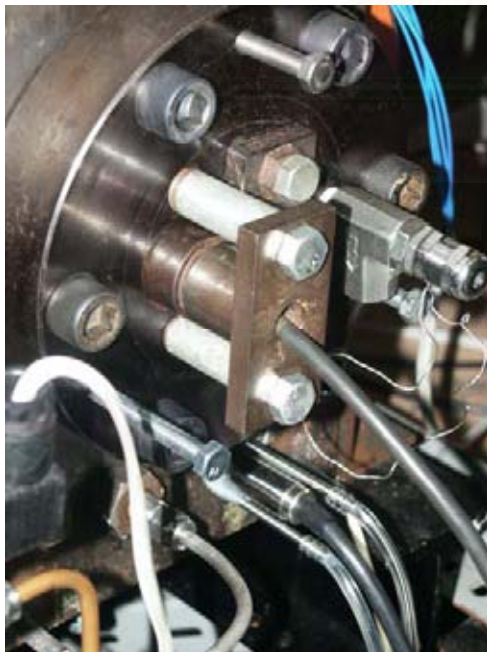
Fig.3-7 Spark plug position at combustion chamber
