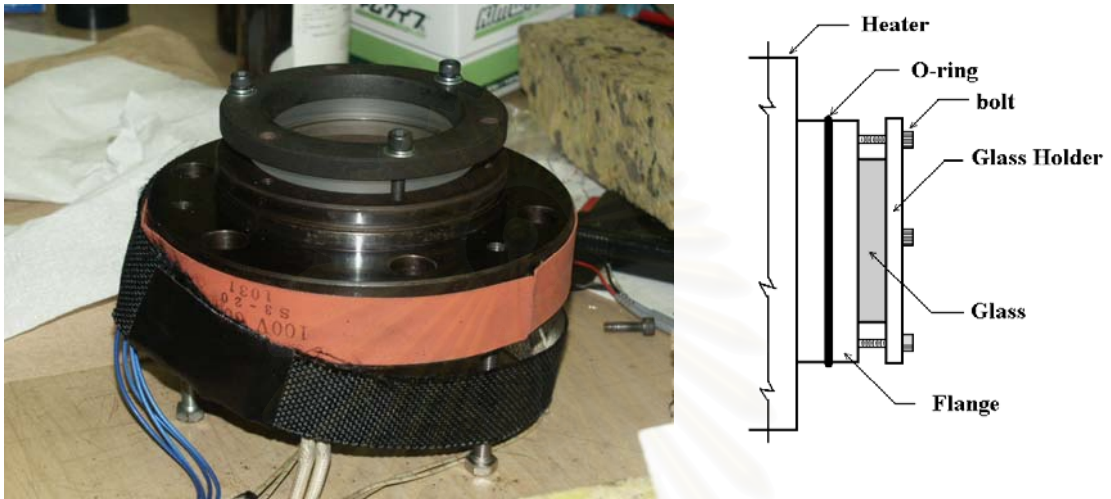
Fig.3-4 Observation window component
