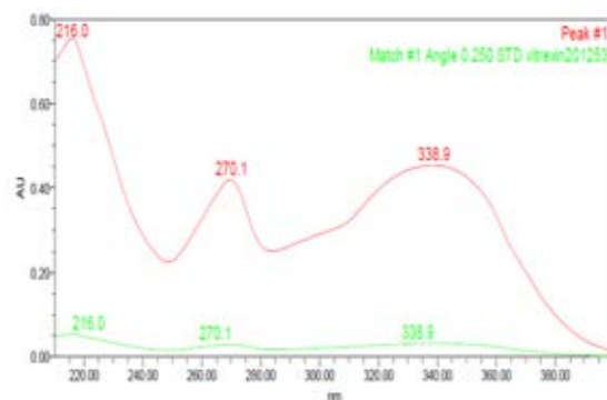
(b) UV spectrum of vitexin after exposure to 1N HCl for 7 days
