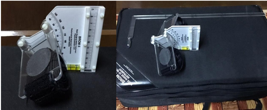
Figure 3.2 The Back Range of Motion (BROM II) shows the inclinometer and an L-shaped slide arm of its flexion/extension unit.
