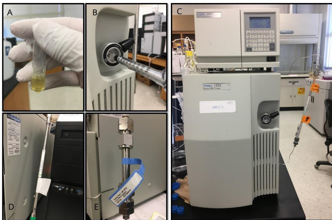
Figure S 1. (A) Reconstituted crude king cobra venom with approximately concentration of 50 mg/mL. (B) Loading knob of the HPLC machine. (C) binary HPLC system (Waters® 1525) and the UV/Vis light detector (Waters® 2489). (D) C18 column for RP-HPLC (Grace® Vydac 218TP™). (E) SP 5W column for the cation exchange chromatography (Waters® Protein Pak™).
