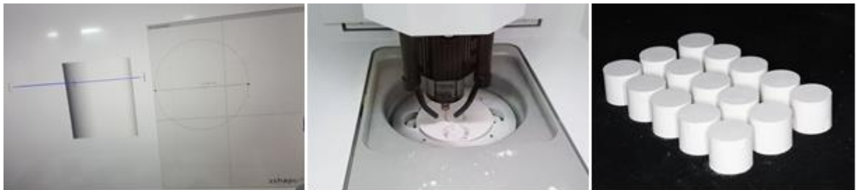
Figure 5 The specimen was designed and milled by CAD-CAM software
