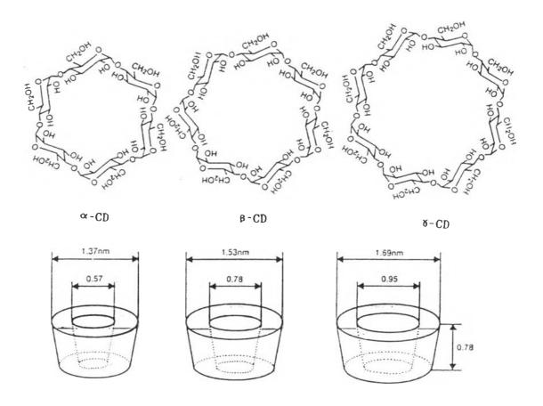
Figure 1.1 Structure of  $\alpha$ -,  $\beta$ - and  $\delta$ -cyclodextrins (Szejtli, 1988)
