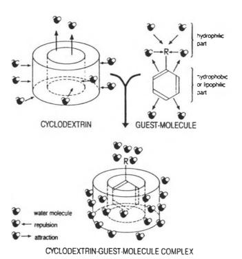
Figure 1.2 Illustration of inclusion of cyclodextrin and guest-molecule (Janssen, 1992)
