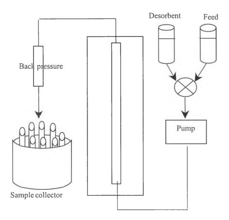
Figure 3.1 The experimental set-up for the dynamic adsorption experiments
