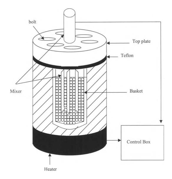
Figure 3.2 The experimental set-up for the equilibrium adsorption experiments
