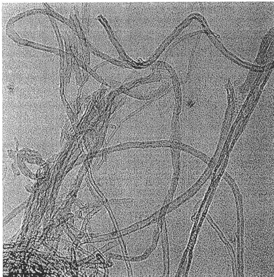
Figure 4.1. TEM image of as-received MWNTs showing the bundles of MWNTs, which are clearly visible, the 10 nm scale is shown in the bottom left corner.
