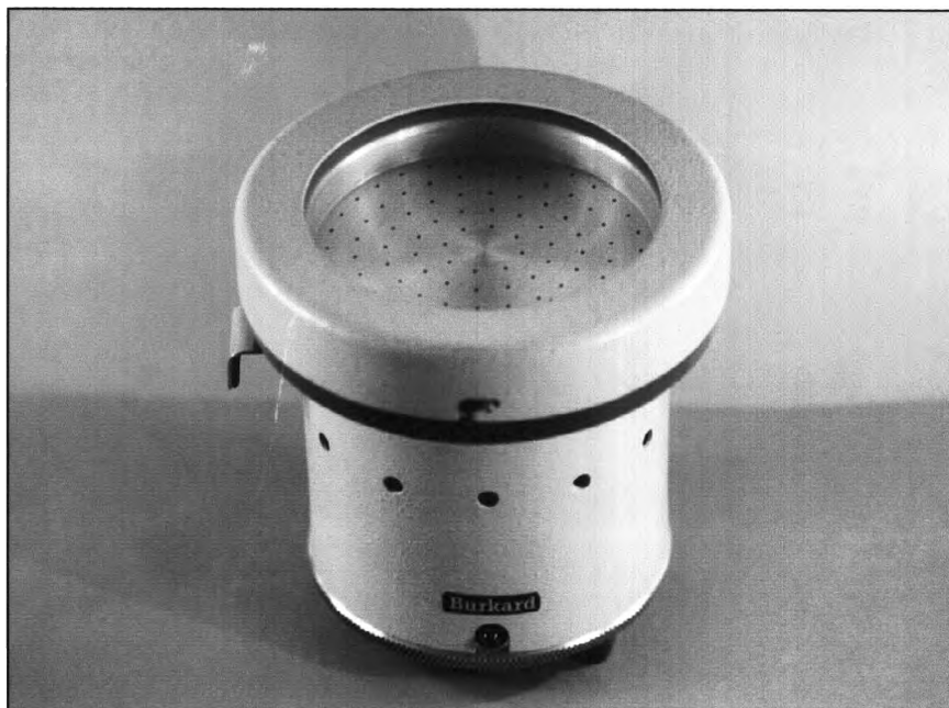
Figure 3.3: The portable air sampler for agar plates.
