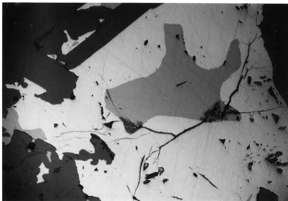
Figure 3.54 Photomicrograph of wollastonite skarn showing an intergrown of chalcopyrite (yellow), bornite (pinkish) and covellite along fracture.
