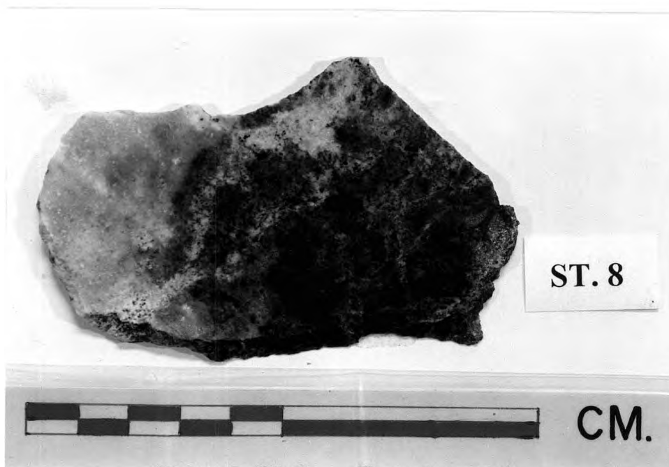
Figure 3.47 A specimen of contaminated diorite containing medium-grained hornblende, clinopyroxene, plagioclase feldspar and fine-grained quartz veinlets.
