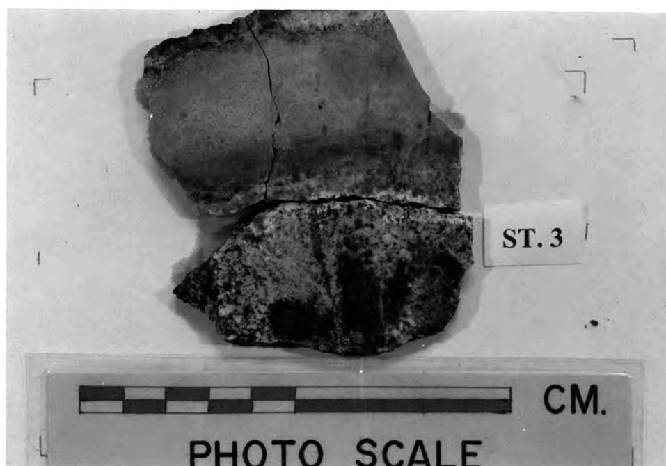
Figure 3.40 A specimen of garnet skarn containing reddish brown, fine to medium-grained type I garnet in contact with contaminated diorite.
