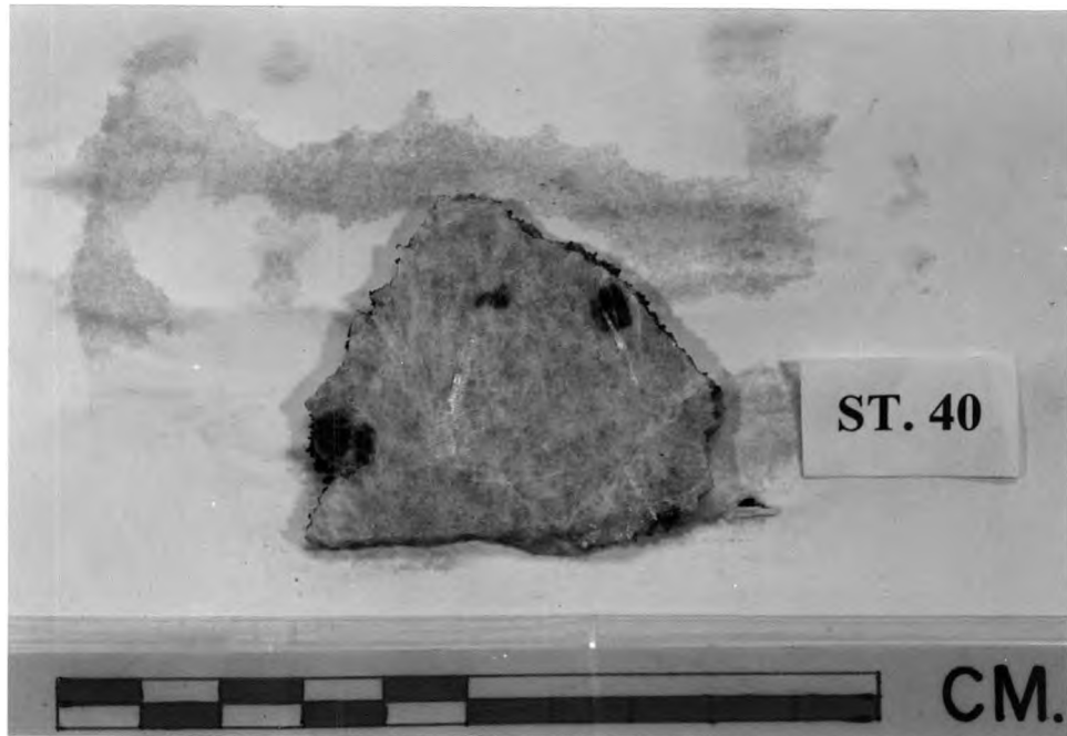
Figure 3.32 A specimen of wollastonite skarn containing coarse fibrous wollastonite (white) and coarse-grained garnet (brown).
