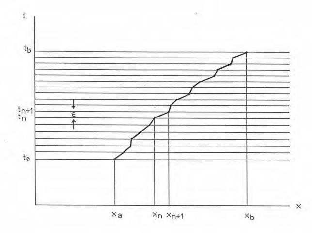
Figure 3.1: The sum over paths is defined as a limit, in which at first the path is specified by giving only its coordinate x at a large number of specified times separated by very small intervals  $\epsilon$ . The path sum is then an integral over all these specific coordinates. Then to achieve the correct measure, the limit is taken as  $\epsilon$  approach 0.
