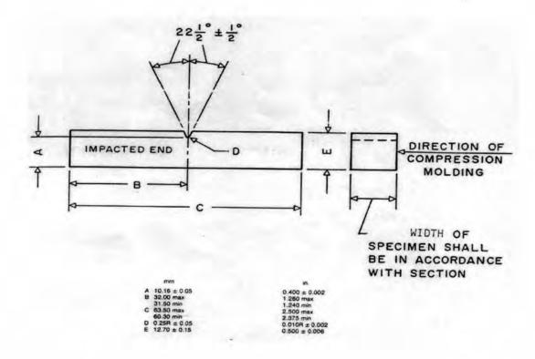
Figure 3.1 Dimensions of Izod-Type Test Specimen [52]
