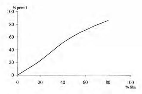
Figure 4-1: Printing characteristic curve of offset print, using the original map image data
