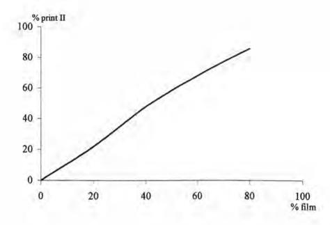
Figure 4-2: Printing characteristic curve of offset print, using the output data from the RTSDZIP
