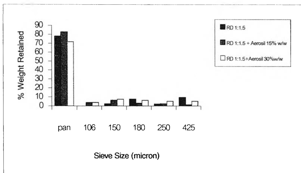
Figure 24 Particle size distribution of spray dried diclofenac sodium with Eudragit® RD 100, with the aid of Aerosil® 200 = 0, 15, 30 % w/w at the same ratio of 1:1.5.
