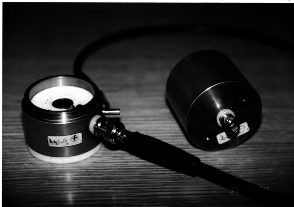
Figure 2.2 The pellet sample holder for impedance measurements.
