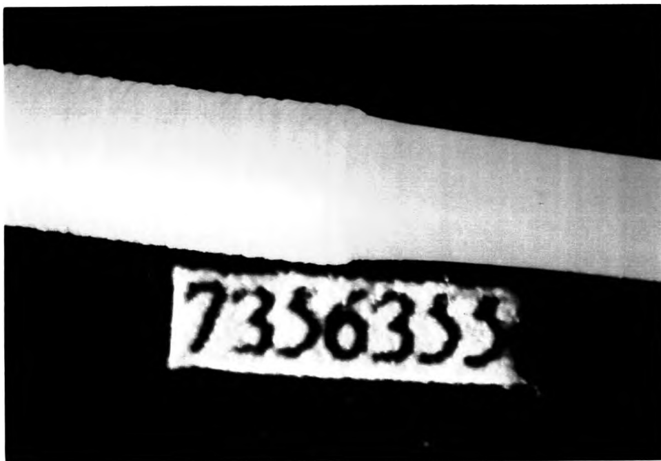
Figure 3.23a Stereomicroscope photograph of a ripple/hazy smooth extrudate in the oscillating regime at HDPE/PP(P340J) : 70/30. ( \gamma_a = 539.1 1/sec)
