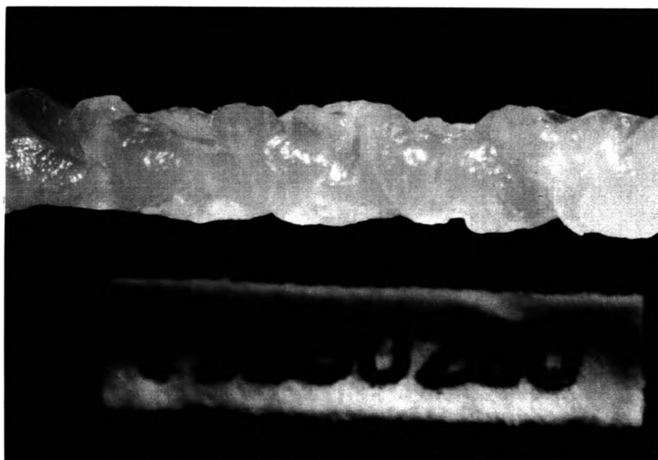
Figure 3.15 Stereomicroscope photograph of the melt fracture extrudate at HDPE/PP(P340J) : 100/0. ( \dot{\gamma}_a = 541.4 1/sec)
