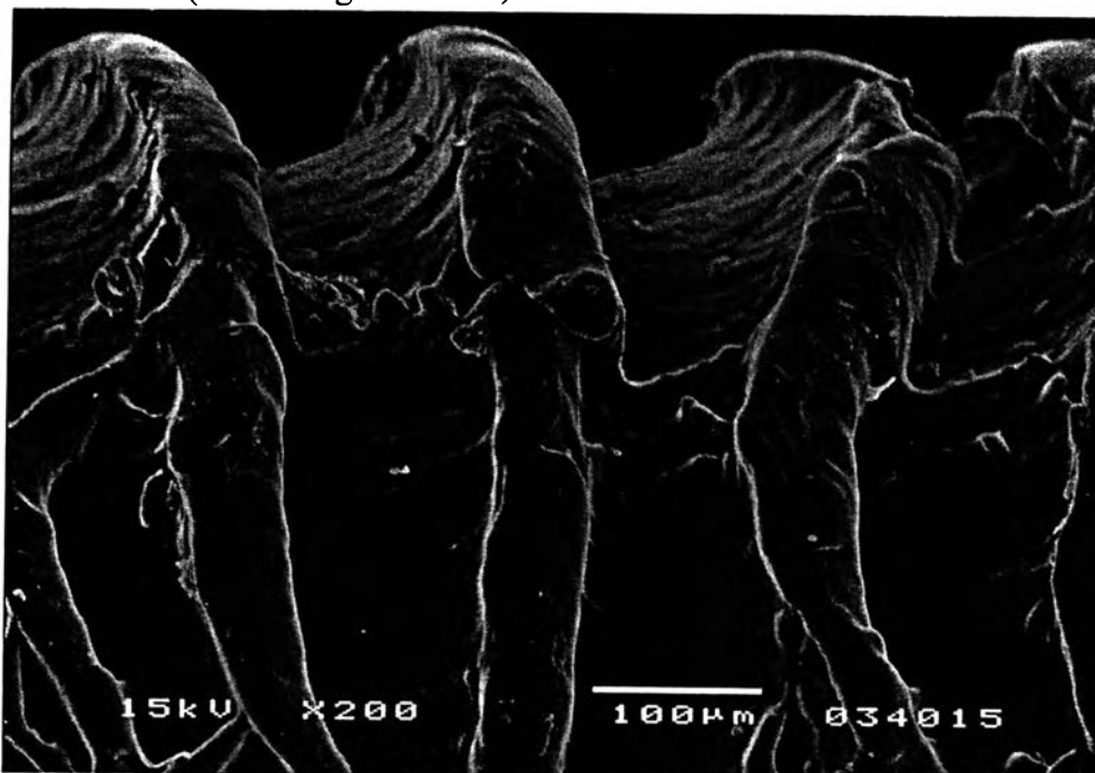
Figure B8 Sharkskin extrudate of HDPE (H5690S) of regime III at 180°C (200x magnification).
