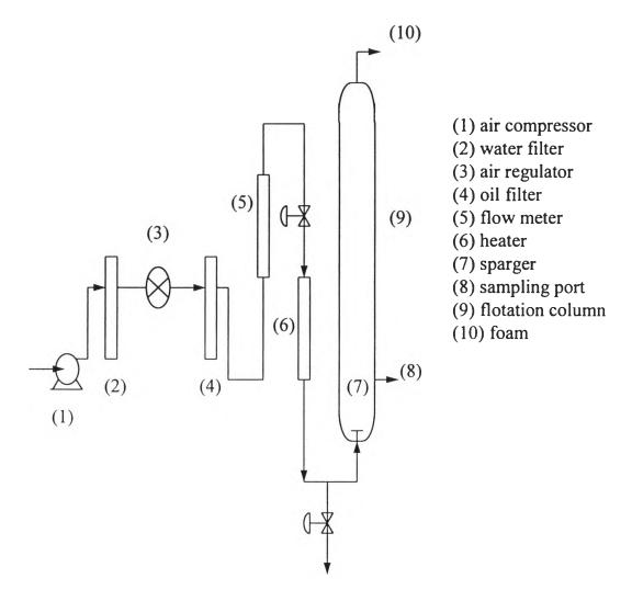
Figure 3.2 Schematic diagram of the experimental apparatus.
