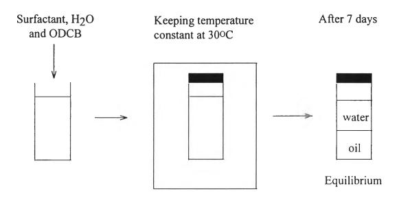
Figure 3.1 Schematic experiment of microemulsion formation.
