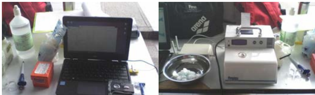
A set of equipment for muscle oxygenation and blood lactate measurement
