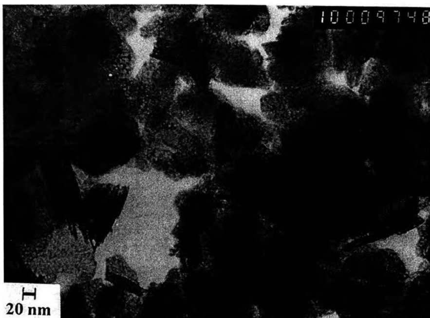
Figure 4.19 TEM micrograph of 0.12 wt.% Au/NiO calcined at 300°C
