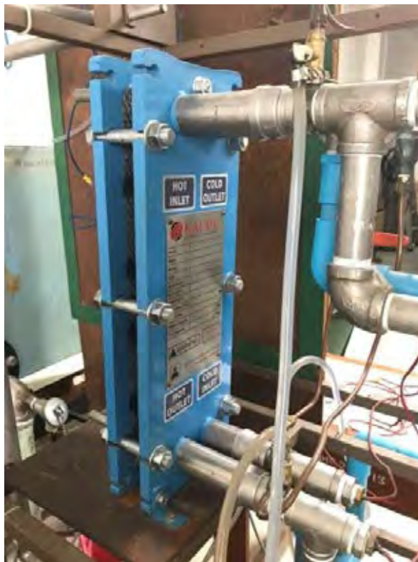
Figure 13 KAUDY, M2 plate heat exchanger installed in a test rig
