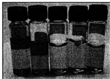
Figure 3.3 Sugarcane bagasse hydrolysates obtained from microwave/chemical pretreatment.
