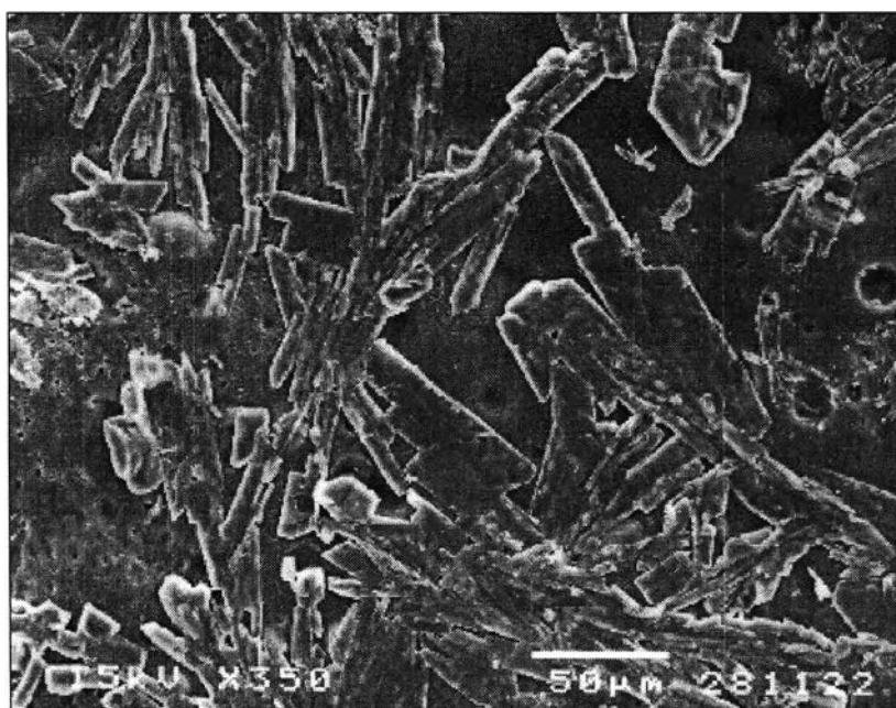
Figure 46 Surface topography of the HPMC:EC film at the ratio of 8:2, containing diltiazem hydrochloride and N-methyl-2-pyrrolidone.
