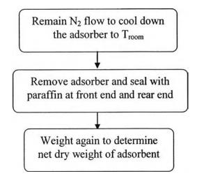
• Adsorption step procedures followed this diagram below;
