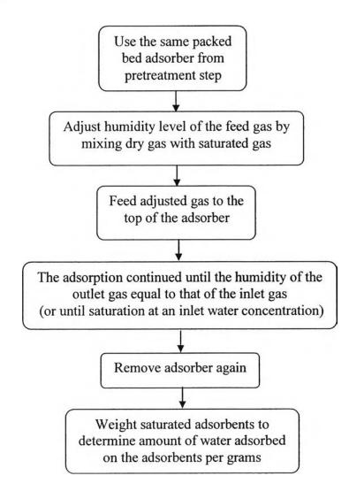
The amount of water adsorbed on the adsorbents per gram was calculated as follows;
