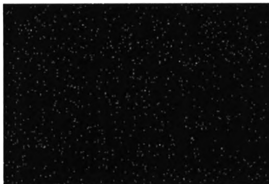
Figure 4.19 SEM-EDX images of Zn atom distributed on NR/ZnO-coated DBD plasma-treated cellulose surface.
