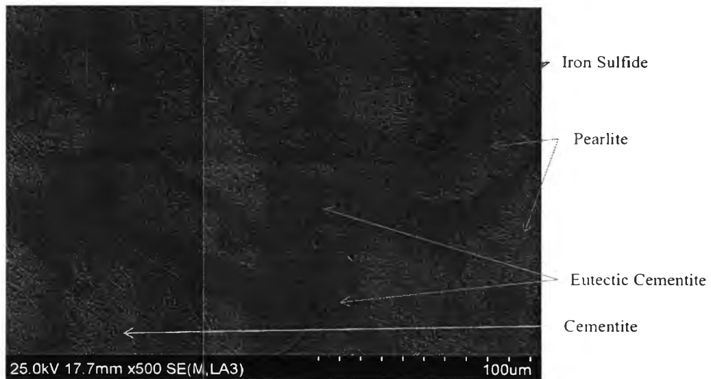
Figure 6 The backscattered SEM image of cross section iron nugget No. 3.4 at reduction temperature 1,425°C and reduction time of 20 min. The lamellar structure represents pearlite, which is alternating layers of \alpha iron and Fe 3 C, light-gray areas represent cementite (Fe 3 C) and dark-gray areas represent the iron sulfides. This structure is similar to the white cast iron.
