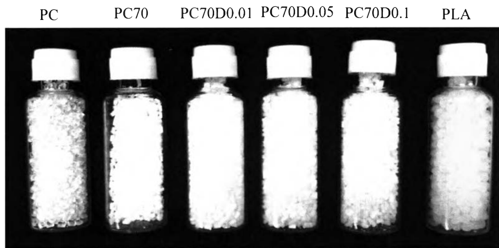
Figure 5.2 Pellets of PC, PLA and uncompatibilized PC/PLA/DBTO blends.
