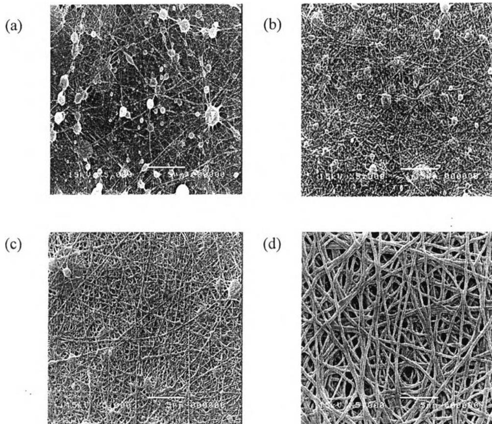
**Figure 3.1** SEM images of electrospun SF fibers at different concentrations: a) 10%, b) 20%, c) 30%, and d) 40% (w/v). The EFS was applied at 20 kV/10 cm. (magnification = 5000x, scale bar = 5  $\mu$ m)
