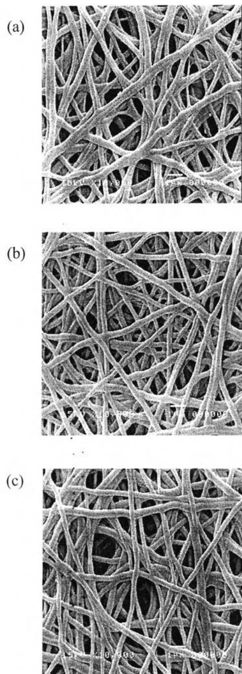
**Figure 3.2** SEM images of electrospun SF fibers from 40% (w/v) SF solution after methanol treatment at different applied EFS: a) 15 kV, b) 20 kV, and c) 25 kV/10 cm. (magnification = 10000x, scale bar = 1  $\mu\text{m}$ )
