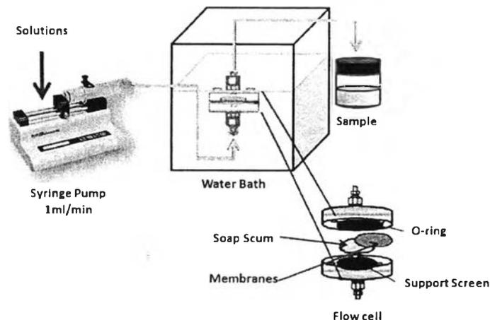
**Figure 3.1** Flow cell apparatus.
