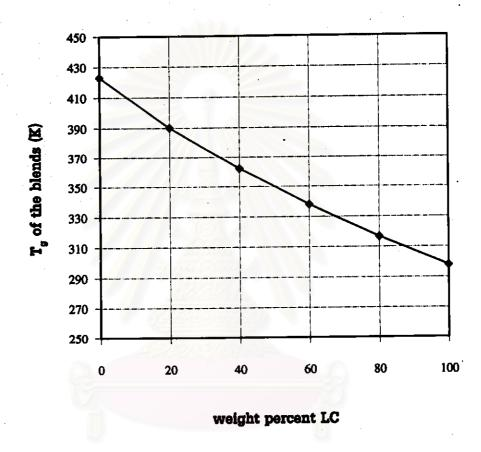
**Figure A-1** The graph of the glass transition temperatures  $(T_q)$  of the blends against the weight percent of low molar mass liquid crystal.
