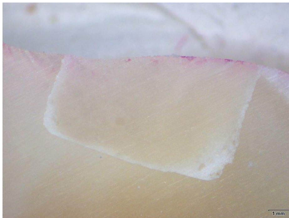
Figure 2 No leakage at tooth-resin interface (arrowed) of 1-1 primerless wet bonding of 4-META/MMA-TBB resin adhesive in 1-1 30 seconds group
