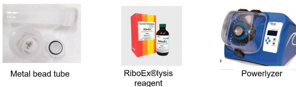
Figure 7 Reagent and device used for bone homogenization
