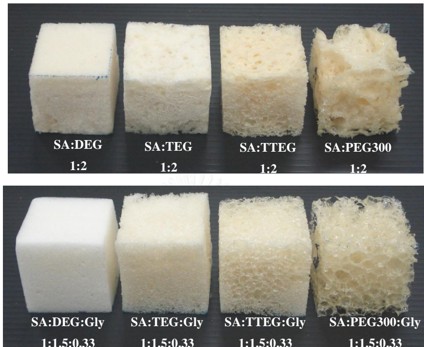
Figure 4.11 Cubic specimens of bio-based PU foams prepared from SA and neat-glycol polyols (top), PU foams prepared from SA and mixed-glycol polyols (bottom)
