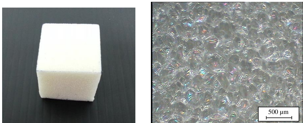
Figure 4.14 Cubic specimen and OM image of the PU foam prepared from SA and commercial polyester polyol (A8360)
