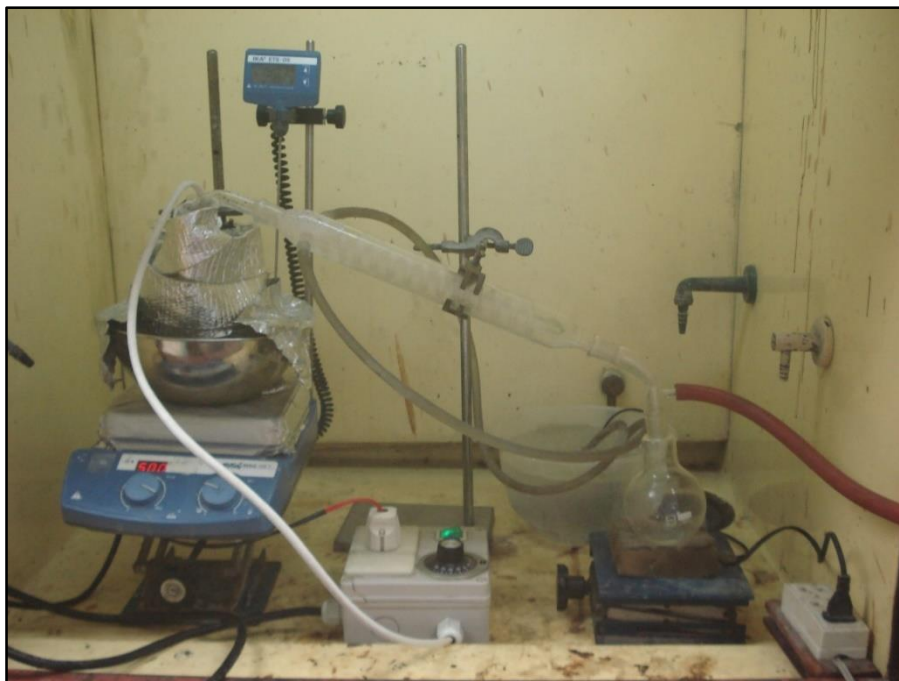
Figure 3.2 The experiment set up for the synthesis of bio-based succinate polyols
