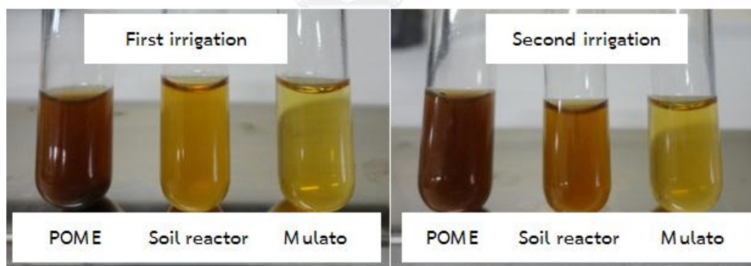
Figure 4.15 Comparison of color of the leachates from soil reactor and Mulato rhizoreactor in the first and second irrigation cycles.
