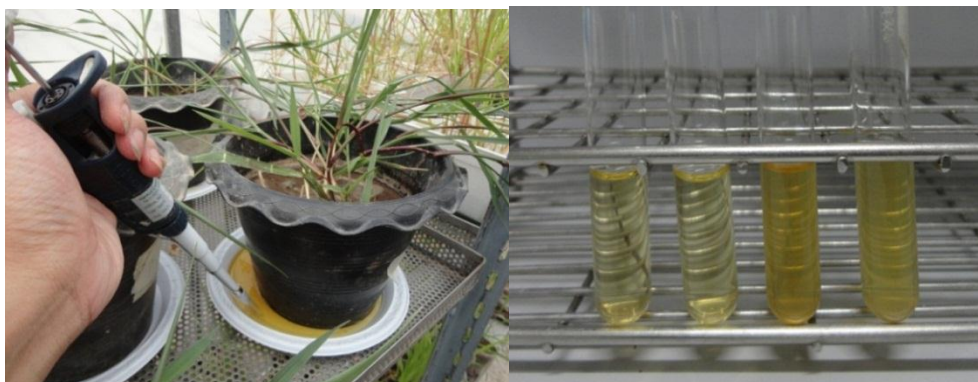
Figure 3.9 Water leachate collection from grass pot
