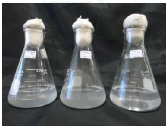
Figure 3.5 Phenol degradation test in CFMM containing phenol 100 and 500 \text{ mg L}^{-1} phenol and control.
