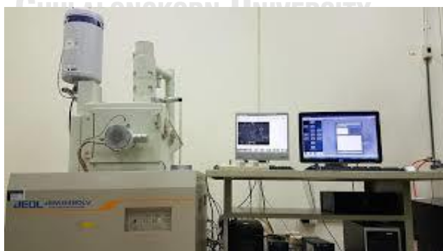
Fig. 3.1 Scanning Electron Microscopy with Energy Dispersive Spectroscopy (SEM-EDS) (JEOL, model JSM-5480LV)
