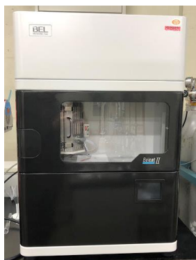
Fig. 3.6 Chemisorption analyzer (MicrotracBEL, model BELCAT II).
