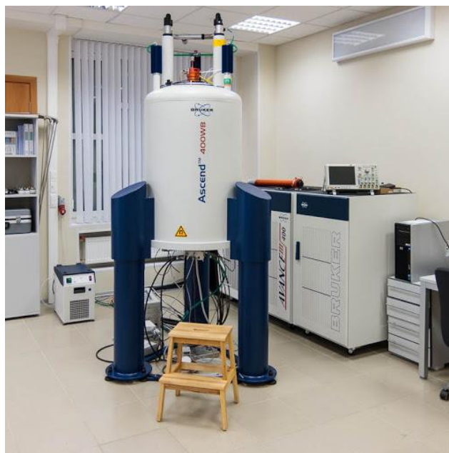
Fig. 3.5 Nuclear magnetic resonance spectrometer (solid state - NMR) (BRUKER, AVANCE III HD-Ascend 400 WB).
