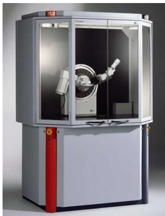
Fig. 3.4 X-ray diffractometer (XRD) (Bruker, model D8 advance)
