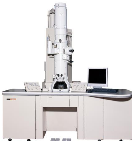
Fig. 3.3 Transmission electron microscopy (TEM) (JEOL, model JEM1400)
