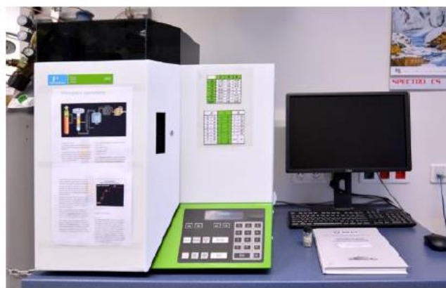
Fig. 3.10 CHN analyzer (model PE 2410, PerkinElmer).
