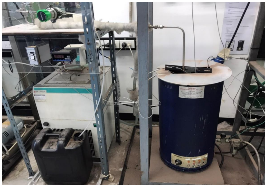
Figure 3.4 The continuous reactor (tubular reactor) which compact in fluidized sand bath and equipped with cooling system
