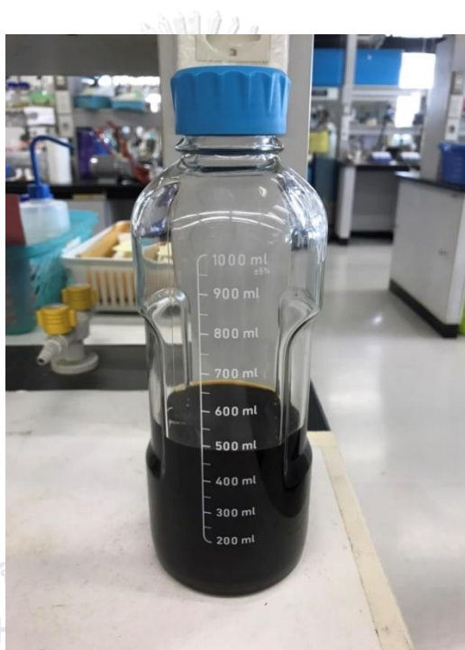
Figure 3.2 The mixture of coffee oil and ethyl acetate after filtrated the SCGs
