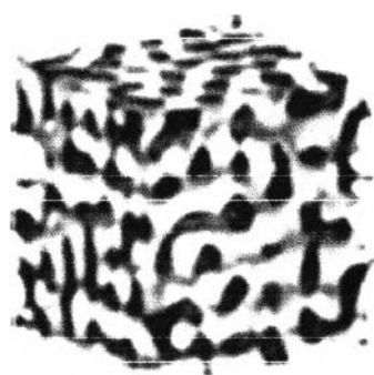
Figure 2.3 Three-dimensional pore systems of TUD-1. (Angevine et al. , 2009)
