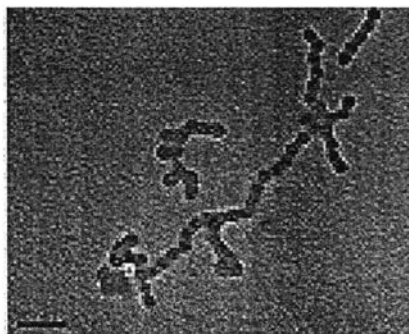
Figure 2.3 The pearl-necklace-like” morphology of micelle PS- b -PEO associated PAA.
