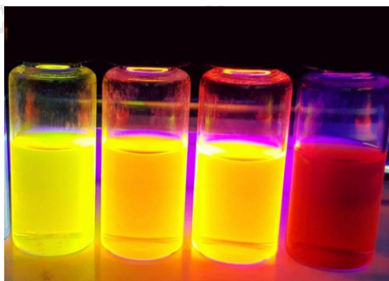
Figure 4.1 The synthesized CdSe/ZnS core/shell QDs with difference sizes in hexane under a UV lamp.
