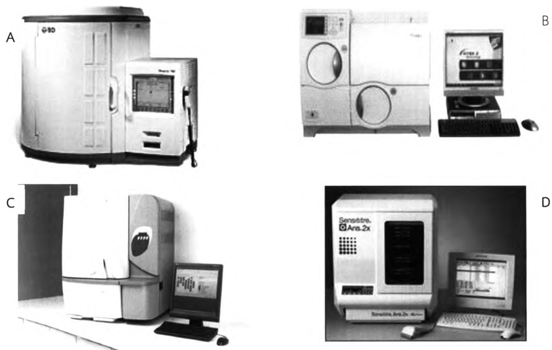
Figure 5 Automated instrument systems are (A) BD Phoenix Automated Microbiology System ®a , (B) Vitek 2 System ®b , (C) MicroScan WalkAway ®c , (D) Sensititre ARIS 2X ®d .
