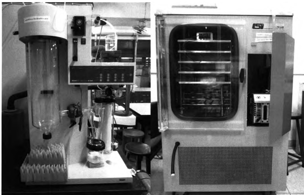
Figure 62 BUCHI mini spray dryer (left) and Freeze dryer (LYOLAB) (right)
