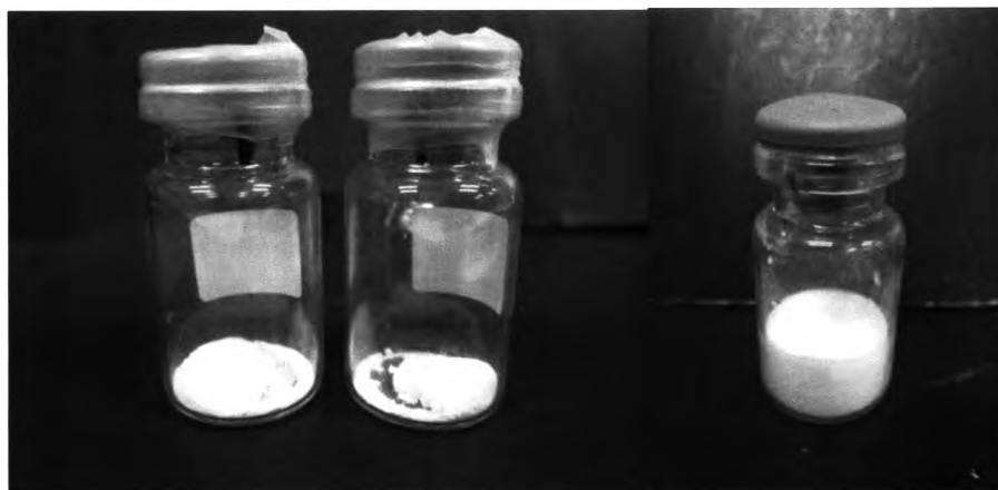
Figure 71 Spray dried RA microparticles (left), freeze dried cake (right)
