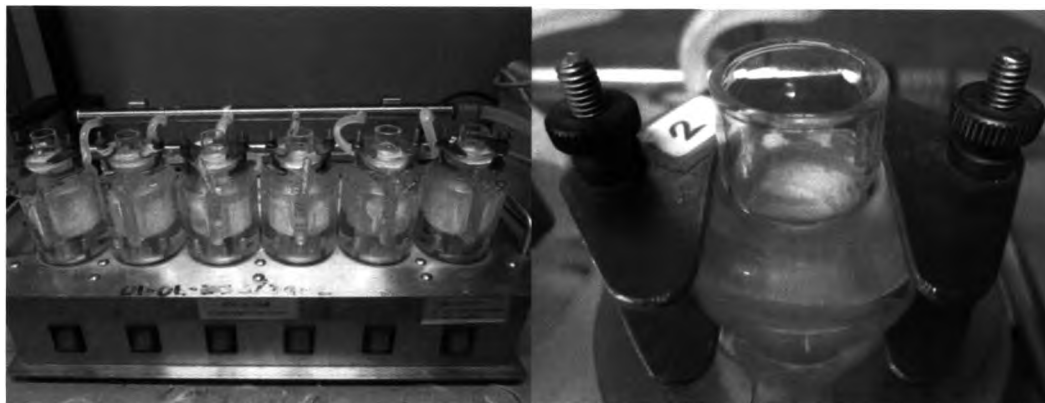
Figure 79 Franz diffusion cell (left), TC MPs-loaded patch release study using Franz diffusion cell (right)
