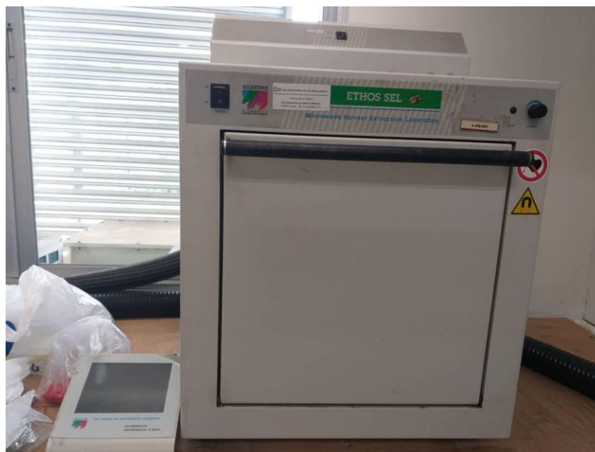
Figure 3.15 Microwave digester (Milestone, ETHOS SEL)
