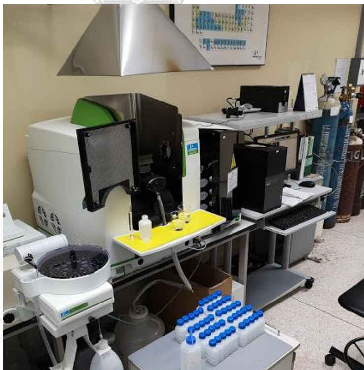
Figure 3.16 Graphite Furnace Atomic Absorption Spectrometry (The PinAAcle™ 900 Serie of AA Spectrometers, PerkinElmer®).
